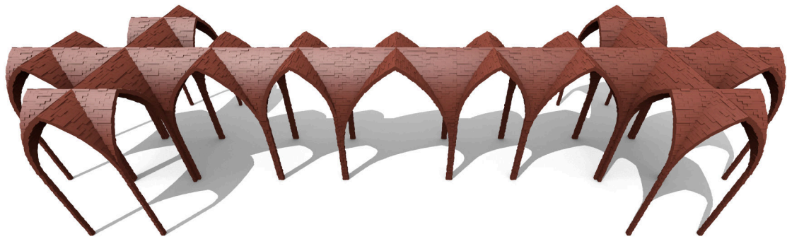
Figure 6.9.: The cross vault from Figure 6.7 can be easily repeated to form gangways. The length and width of a procedural cross vault are independent, which allows them to be combined in interesting ways. Additionally, the bricks have been modeled with repeat splits.
