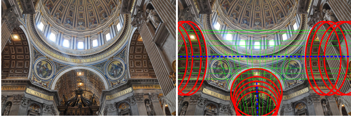
Figure 3.2.: Interior image of the St. Peter's basilica (left). The elements at the arches are arranged circular and those at the dome spherical. The arrangements of these elements have their own reference coordinate systems. For the arches the two cylindrical coordinate systems are depicted (right). The blue lines depict the main axis. For the generation of the coffers, possible splits along the axis are depicted in red, and possible splits circular around the axis are depicted in green. Image taken from [1].
