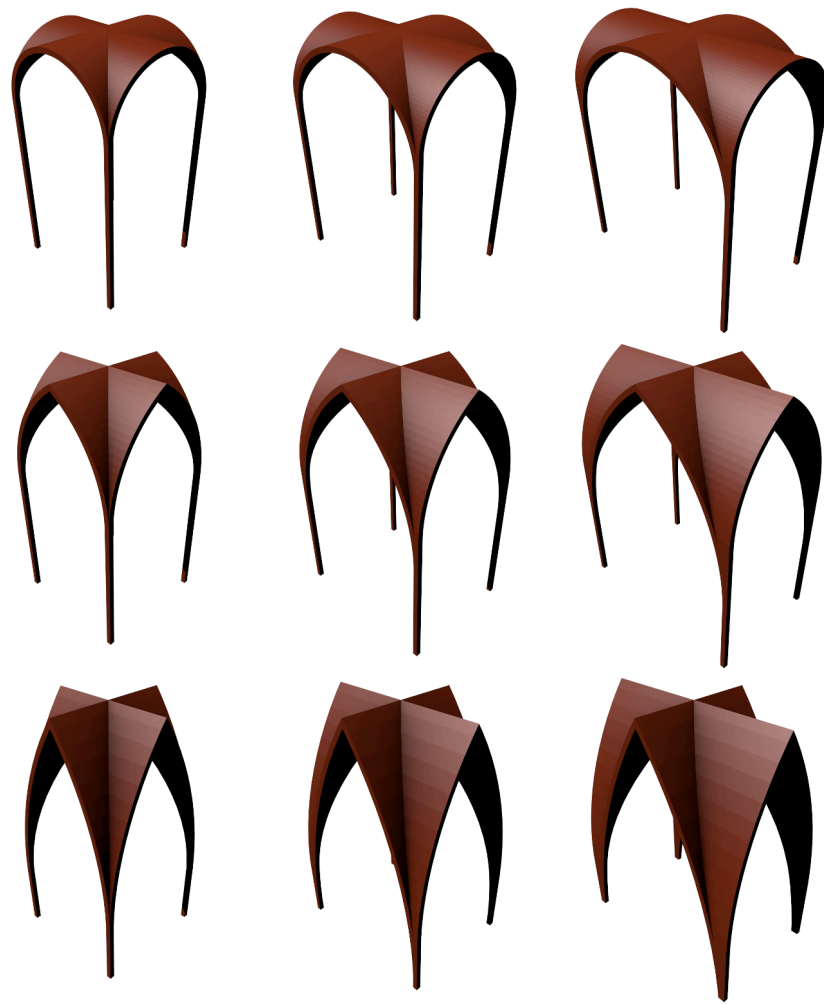
Figure 6.7.: Variations of a procedural cross-vault model. To the right the width increases, and the arch automatically adopts to the new space. To the bottom the angle of the arch decreases and the arch becomes a pointed arch.
