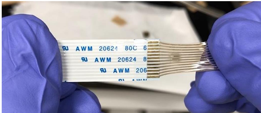
Figure 7.3 Photograph of the PSA bonding between an Au-PDMS conductive film and an FFC (flexible flat cable), showing strong bonding between the two connectors.
