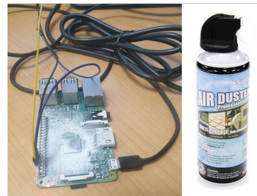
Fig. 2. Demonstration of Raspberry Pi model B+ (Left) frozen by air duster (Right)
