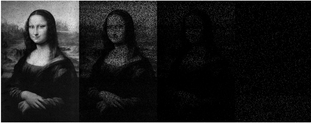
Fig. 3. A MonaLisa image is stored to SDRAM. After powering off for 5 seconds (leftmost), 30 seconds, 60 seconds, 5 minutes (rightmost) at -30^{\circ}\text{C} , the image is recovered via cold boot attack. The leftmost image is indistinguishable from the original.
