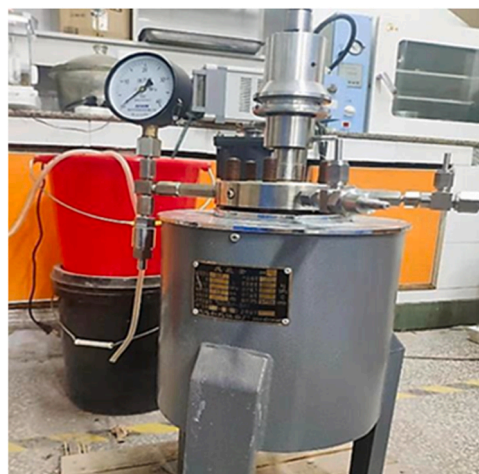
Fig. 1. The diagram of dynamic hydrothermal reactor (GCF).
