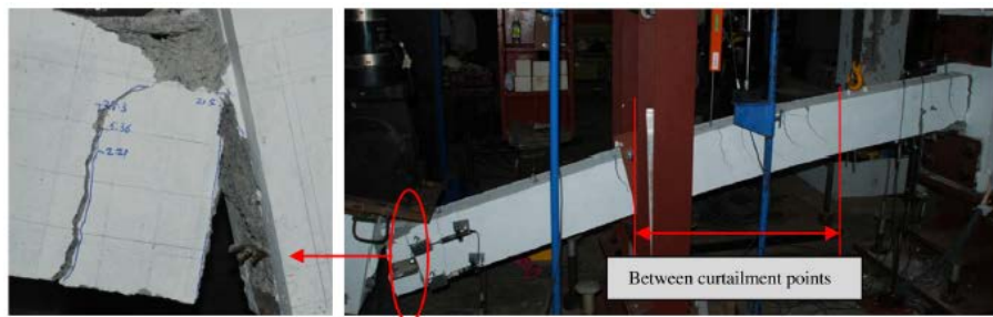
Fig. 2.9: Failure mode of sub-assemblage S1 (Yu and Tan 2013b)
