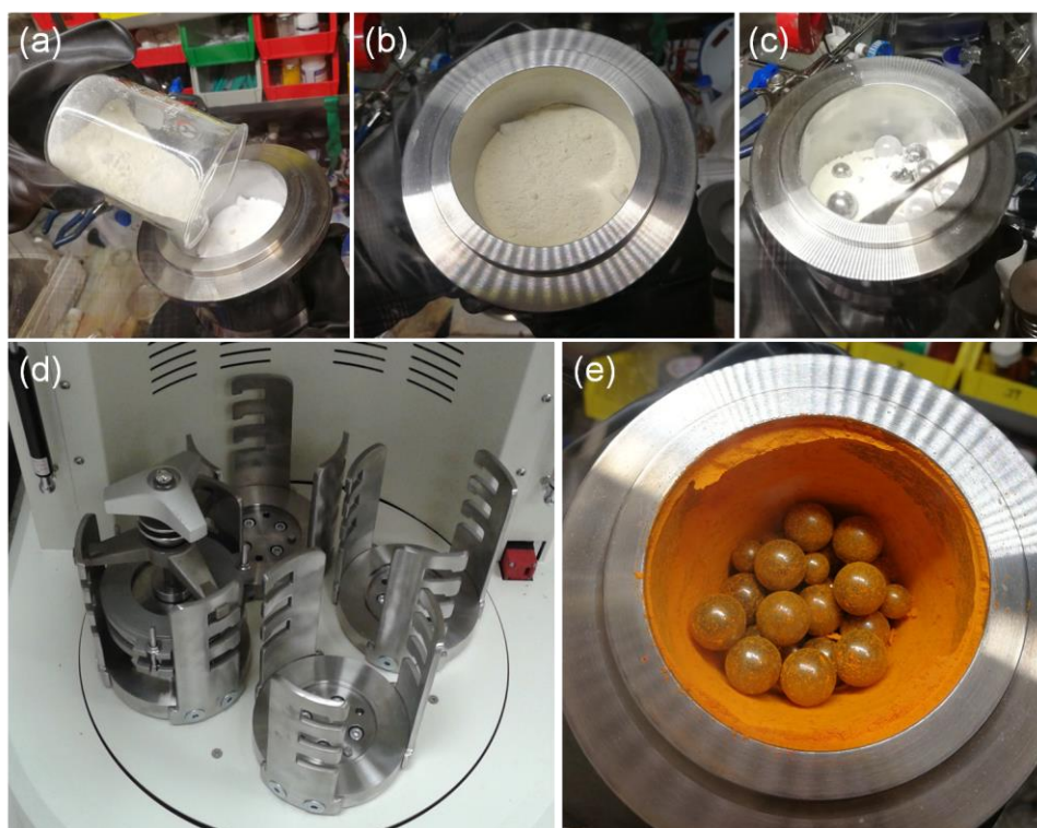
Figure S3. Photographic demonstration of the kg-scale synthesis of \text{CsSnBr}_{1.5}\text{Cl}_{1.5} . a) Preparation of the reagents \text{CsBr} , \text{CsCl} , \text{SnBr}_2 , and \text{SnCl}_2 (all white powders) in a \text{N}_2 glovebox. The reagents were weighed and transferred from a beaker into the 250 mL mechanochemical reaction vessel. The total reagent weight was 250 g. b) The reagent mixture with the milling balls at the bottom of the vessel. c) Gentle mixing of the reagents, which exposed the milling balls, by using a metal spatula. d) Planetary mill containing four reaction vessel holders, essentially allowing four 250 g reactions to take place simultaneously, leading to a 1.0 kg scale batch synthesis of the perovskite. e) The orange product after 10 hr of milling. Related to Figures 1 and 4.
