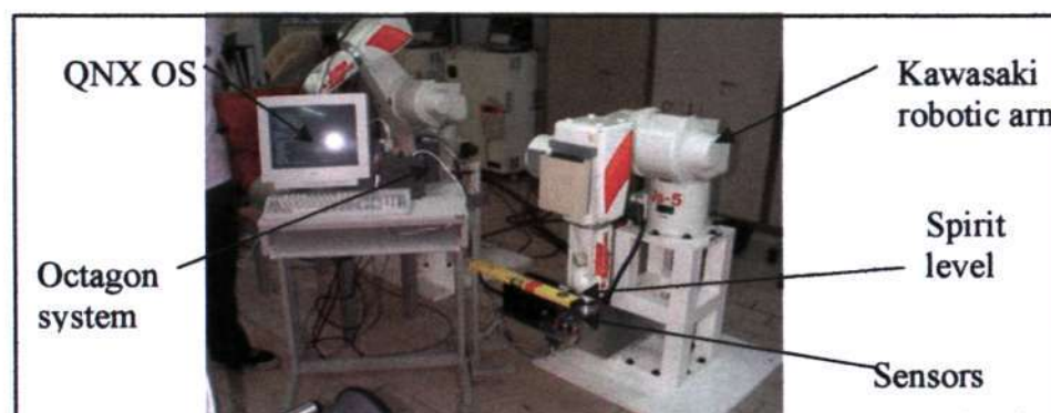
Figure 5.7(b) Kawasaki experimental setup initialisation using a spirit level to test for initial flatness of the end-effector.
