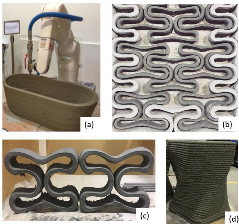
Figure 3: 3D concrete printing research at Nanyang Technological University (NTU), Singapore
