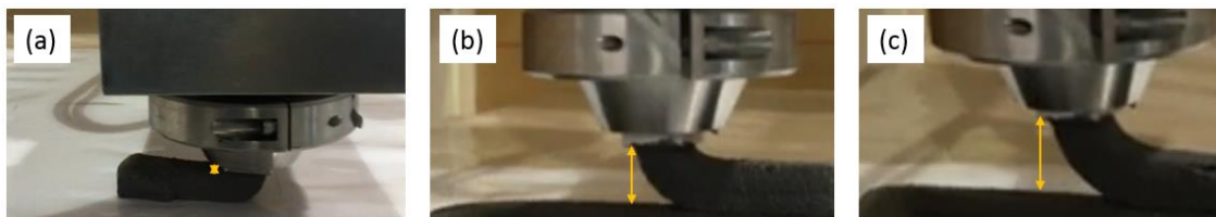
Figure 16. (a) Zero (b) Two (c) Four-millimeter nozzle standoff distances during geopolymer printing
