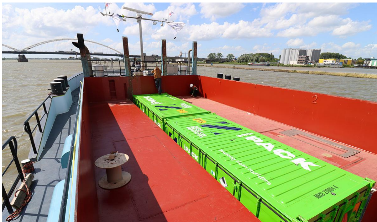
Figure 2-5: Swappable marine batteries in 20-foot ISO containers
