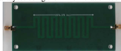
Fig. 1 Fabricated serpentine test sample
