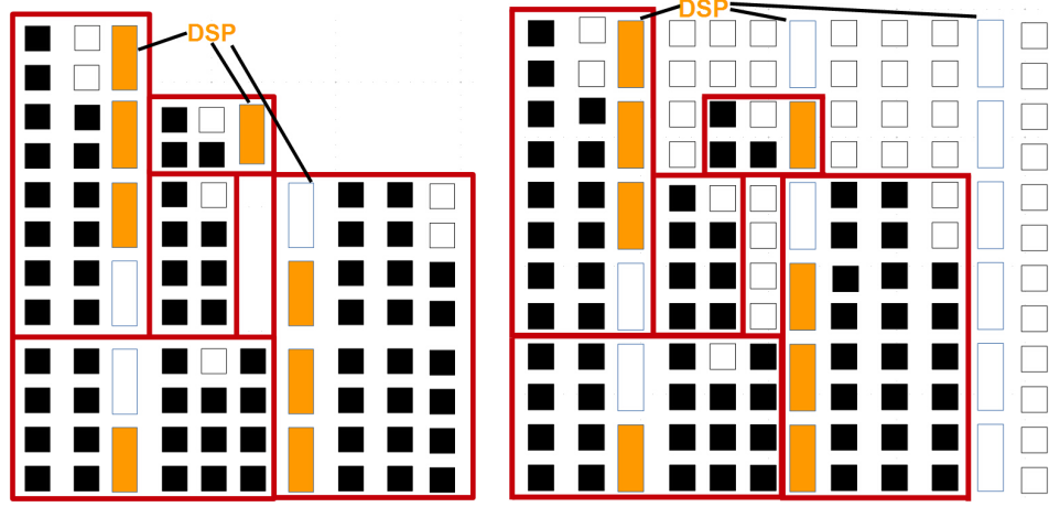
(a) Coarse-grained module placement generated by BMP. (b) Coarse-grained module placement after mapping to the FPGA architecture.
