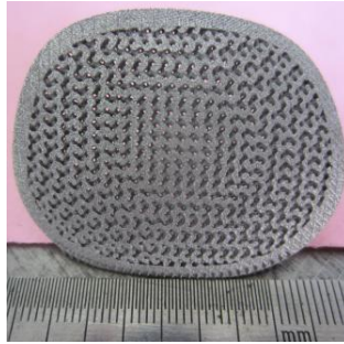
Figure 6. The result of SLM manufacturing porous cranial graft based on implicit surface method
