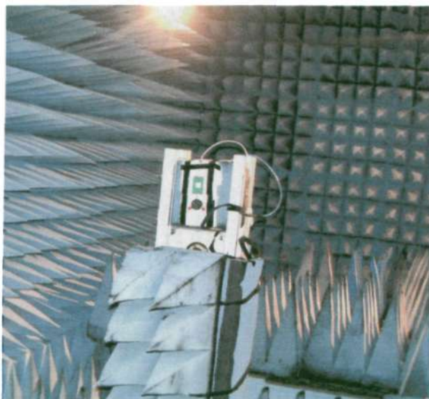
Fig. 4-11 Anechoic chamber room setting up for measuring radiation patterns
