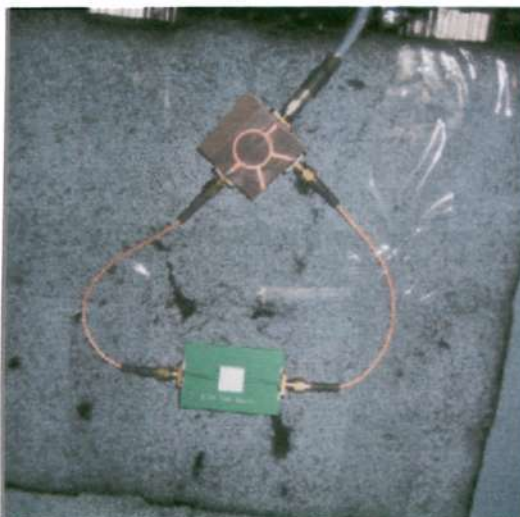
Fig. 6-28 Balun connected with the dual-fed ICPA for measurement
