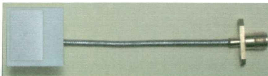
Fig. 3-4 Photo of the fabricated microstrip antenna part of the ICPA for testing
