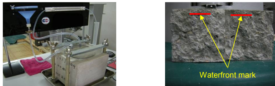
Figure 4.24 Typical setup of initial surface absorption test, showing the waterfront mark after testing
