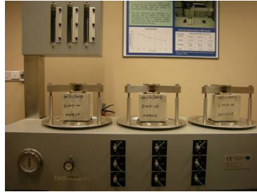
Arrangement of specimens on the testing bays
