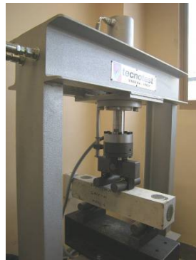
Testing frame for determination of flexural strength of concrete beam
