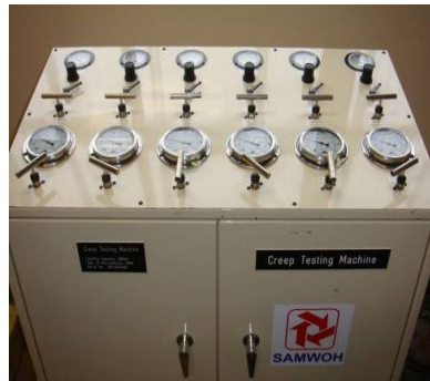
Hydraulic system driven by air compressor
