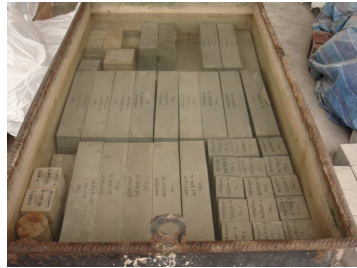
Figure 3.8 Curing condition of hardened concrete specimens
