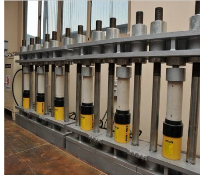
Metal frame for specimen loadings
