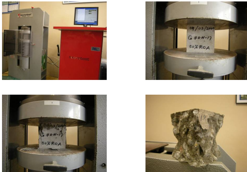
Figure 4.3 Compressive strength test of hardened concrete
