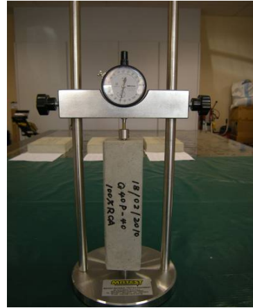
Taking measurement of concrete specimen
