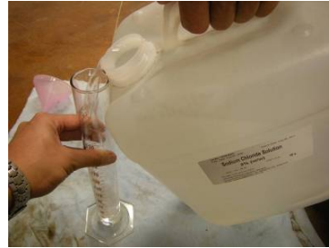
Filling of cells with sodium chloride and sodium hydroxide solution
