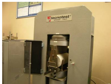
Testing machine with jig for determination of splitting tensile strength
