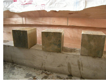
Figure 3.8 Curing condition of hardened concrete specimens
