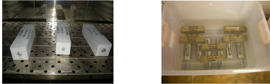
Figure 4.20 Drying with a conditioned oven and wetting in a water bath
