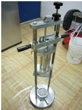
Testing on aggregate impact value of coarse aggregate
