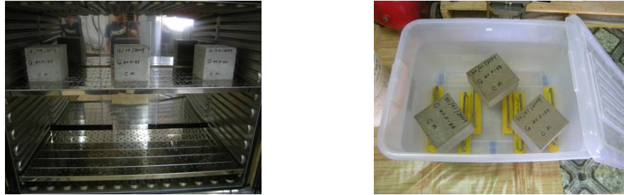
Figure 4.22 Conditioning of specimens for the determination of water absorbability
