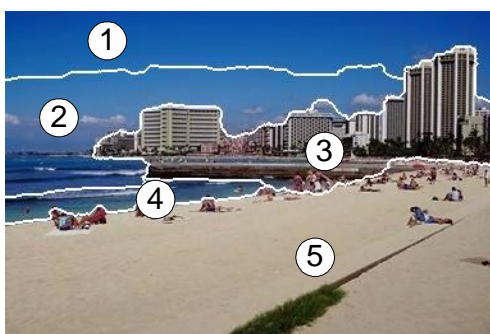
Figure 4.6 - An example of region merging to create a binary tree, five regions created by the segmentation method.
