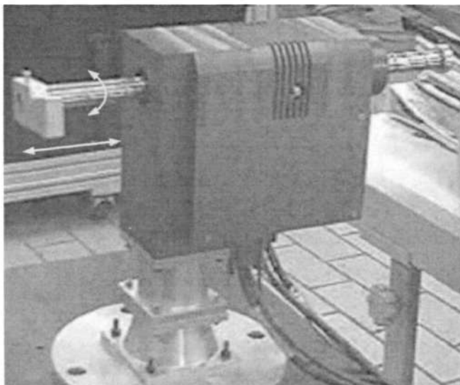
Figure 2.12: The 2-DOF actuator module [76]
