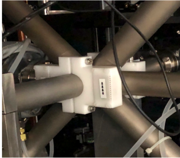
Figure 3.7: Arrangement of permanent magnets for 2D MOT and hybrid bi-color atomic beam slower.
