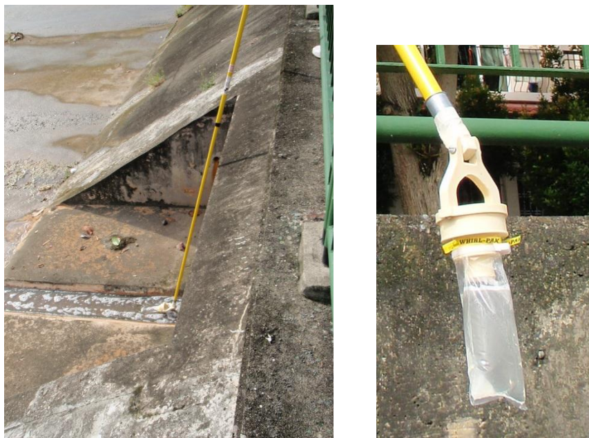
Figure 4.5. The extendable Nasco sampling pole used together with Whirl-Pak® bag
