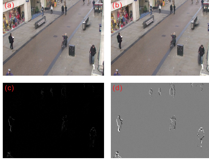
Figure 3.4: “Salt” and “Pepper” noise effect in the temporal difference algorithm. Sub-figures (a) to (d) correspond to the test images inserted with noise, their intensity difference and the motion event image.
