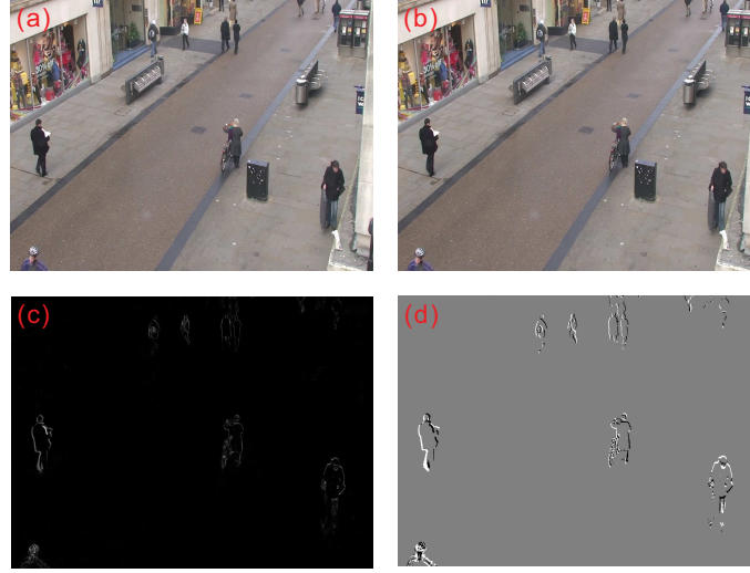
Figure 3.1: Demonstration of the temporal difference algorithm. Subfigures (a) to (d) correspond to two consecutive images, their intensity difference in absolute value and the motion image.
