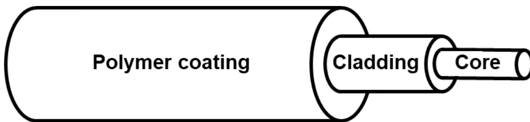
Figure 1.1 Schematic of a basic optical fiber structure.
