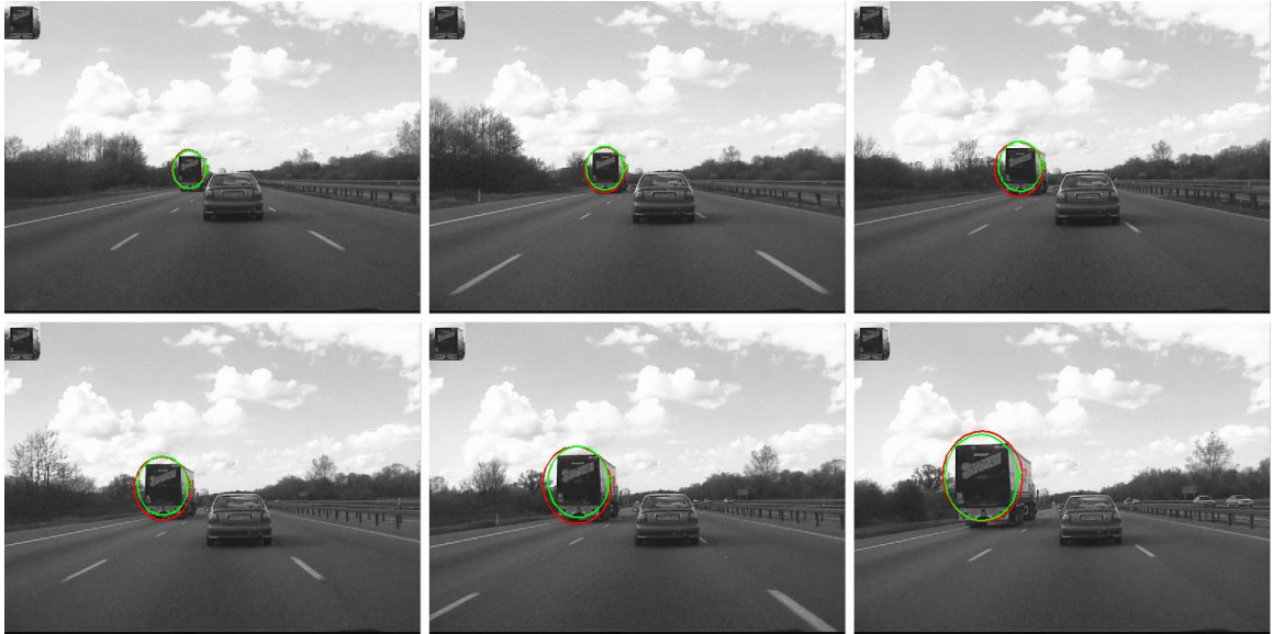
Figure 5.16: Tracking results on PETS2001 vehicle sequences, frame #1, 25, 50, 75, 100, and 125. Green: IPCA, Red: our results. Both results were comparable.
