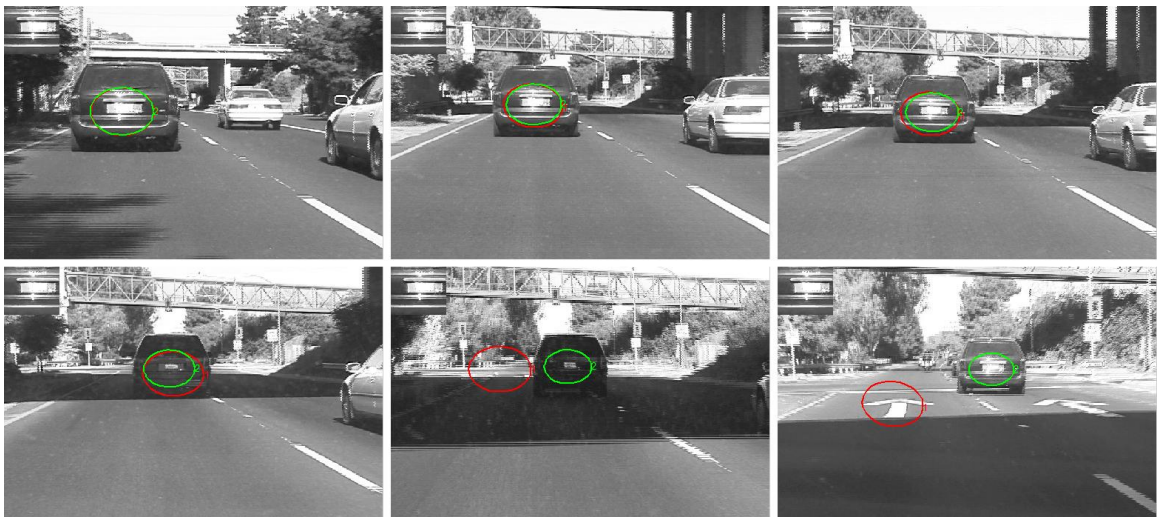
Figure 5.17: Tracking results on car sequences, frame #1, 132, 150, 168, 184, 227, Green: IPCA, Red: our results. The IPCA method performed better and was robust to illumination changes, but our method mainly used template gradients, which changed dramatically due to shadows and lack of reflection of the car plate. At frame #227, the arrow sign might look too similar to the target in gradients.
