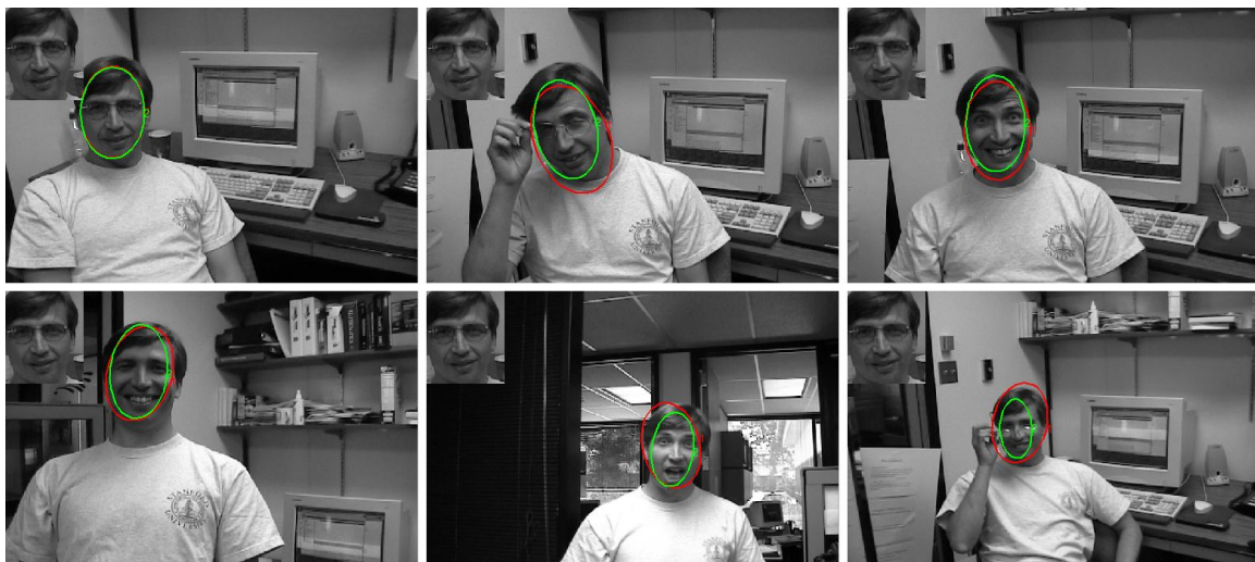
Figure 5.15: Tracking results on DUDEK FACE sequences, frame #1, 361, 459, 605, 795, and 1095. Green: IPCA, red: our results. Both results were comparable despite his rich facial expressions, which had more effect on our covariance descriptor.
