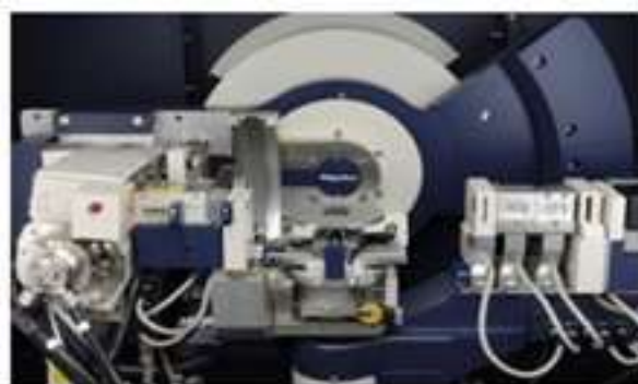
Figure 3.5 Picture of the sample stage of the HR-XRD used in this thesis.
