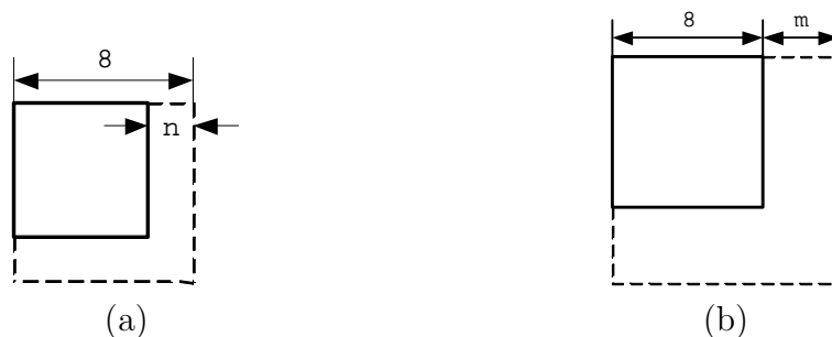
Figure 3.10: 8 \times 8 block based downsampling (a) Sampling ratio (8-n)/8 ; (b) Sampling ratio 8/(8+m)
