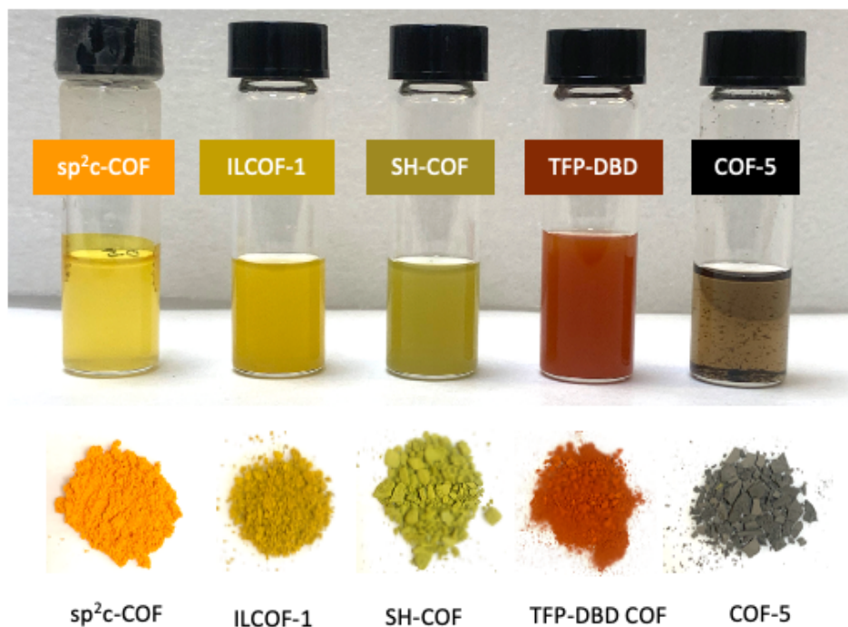
Figure 6.9 Photographic image of the pyrene-based COFs ( sp^2c -COF, ILCOF-1 and SH-COF) and model COFs (COF-5 and TFP-DBD COF) as powder and suspended in DMF.
