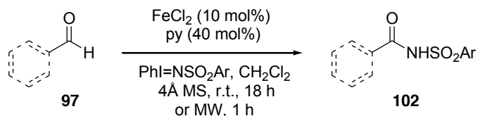
Scheme 2.1 Iron(II)-catalyzed amidation of aldehydes with PhI=NTs at room temperature or under microwave irradiation (MW)
