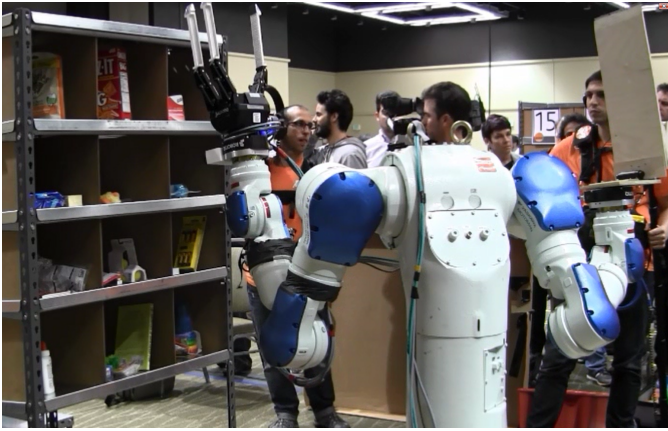
Fig. 4. Yaskawa Motoman with a Robotiq 3-fingered hand with custom extensions and scooping mechanism used by the Worcester Polytechnic Institute (WPI) team.
