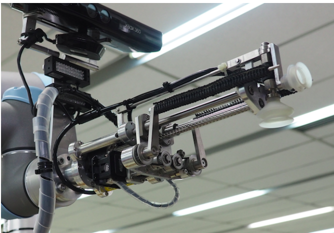
Fig. 6. Team Nanyang's custom gripper has two suctions and one parallel cylinders (fingers). The choice of suction to use depends on the object position. The fingers, which could extend forward and downwards, are used mainly for objects with organic shape.
