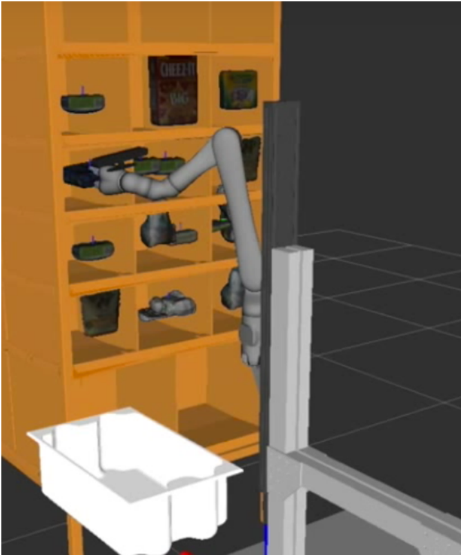
Fig. 10. Team PickNick’s system modeled in the MoveIt! framework [19] that allows access to large variety of path planning tools and visualization.
