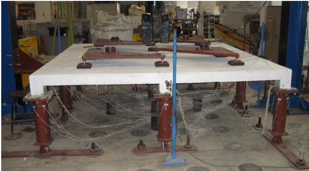
Fig. 16: A typical setup for beam-slab systems subjected to a penultimate column loss scenario
