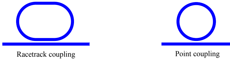
Fig. 2.5. Ring resonators in racetrack coupling and point coupling conditions.
