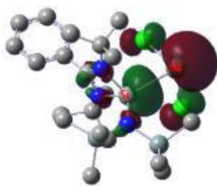
Figure 3.5. HOMO of calculated compound 3.4 showing the donor–acceptor interaction between the Si(II) and Sn(II) centres (isovalue = 0.04).
