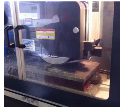
Fig. 4: Grinding machine with water cooling system
