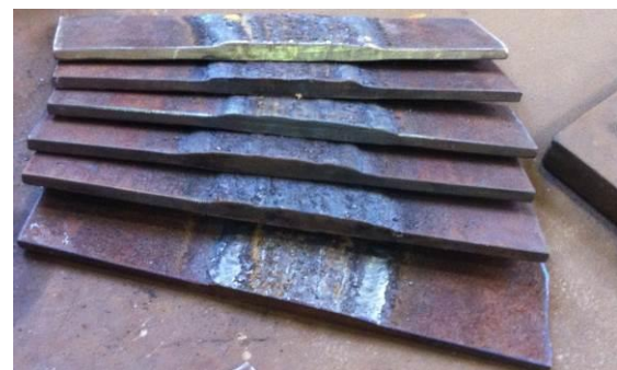
Fig. 3: Coupons cut from the main plate
