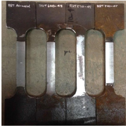
Fig. 5: Final welding affected coupon specimens
