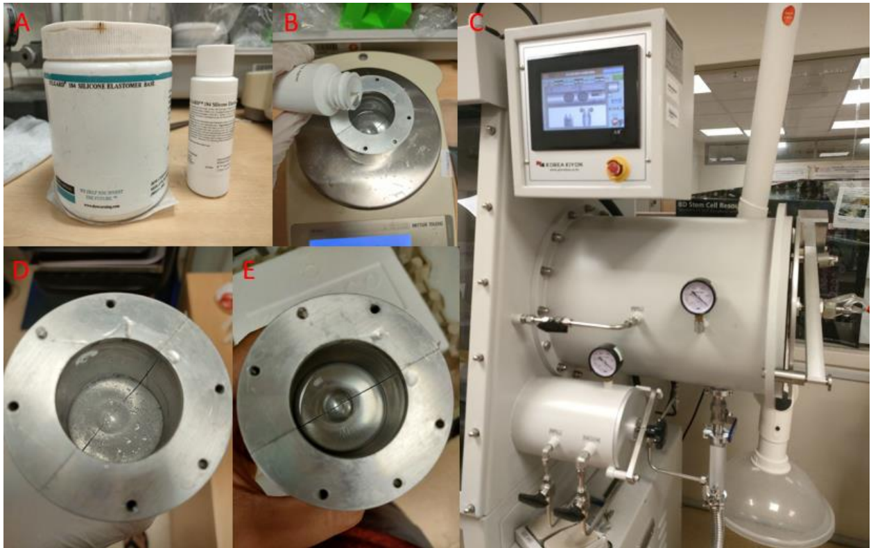
Figure 6: Procedure for curing and preparing the PDMS. A) Image depicting the type of prepolymer and curing agent used (Sylgard-184, Dow Corning, USA). B) Curing agent and prepolymer are mixed thoroughly according to manufacturer's ratio C) Mixture is placed within a vacuum chamber to remove unwanted air bubbles D) Image of polymer mixture before degassing E) Image of polymer mixture after degassing.
