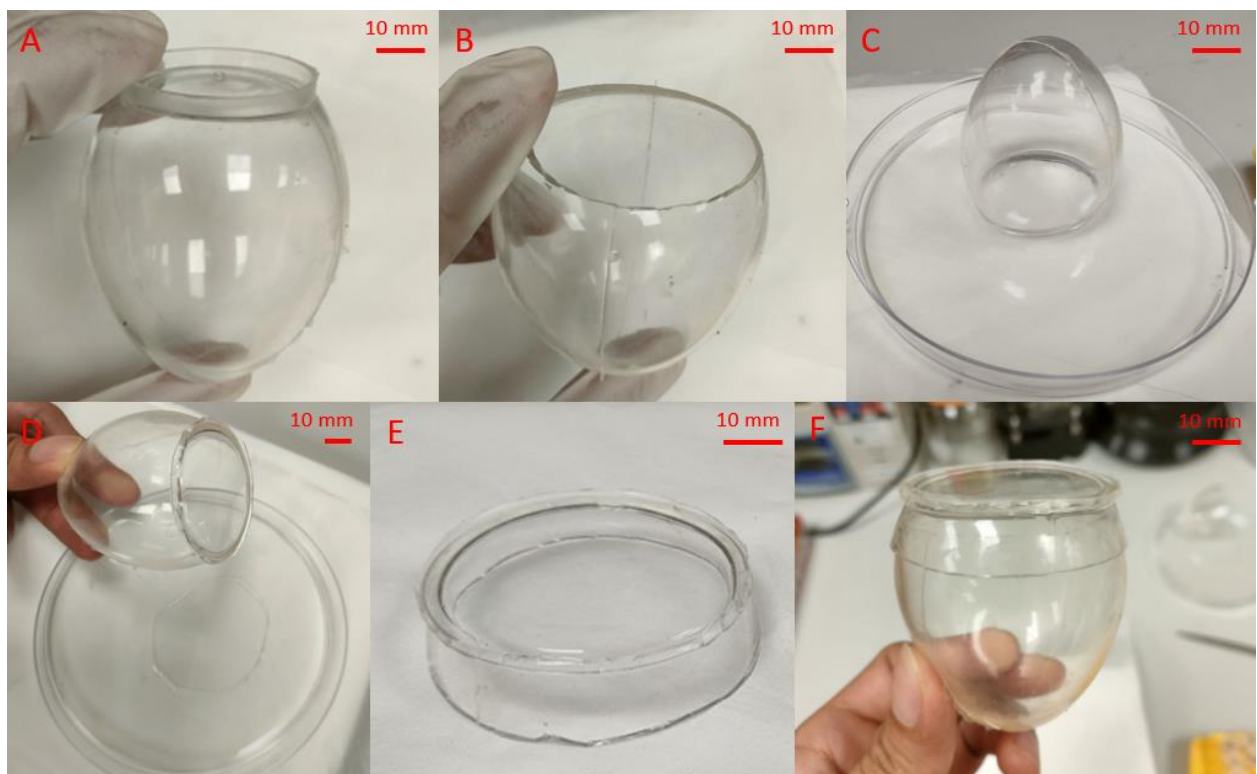
Figure 8: Fabrication process of the ex-ovo PDMS model part two. Requires two PDMS shells for this procedure. A) Raw product obtained after curing treatment and bioreactor process. B) The top of the first PDMS shell is cut off to facilitate an opening for the cover. C) A similar incision is made for the second shell, and it is placed in a petri dish with the same mixture formulation. D) Shell with the newly formed cover component is removed after curing. E) Top portion of the second shell is separated from the body to form a small, cap-like structure, which serves as a cover. F) Cover is placed on top of the first shell to conclude the assembled model.
