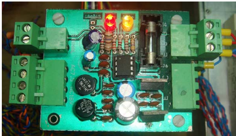
Fig. C.2. Driving circuit for single IGBT
