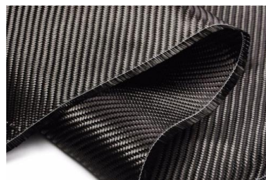
(b) Woven carbon felt (thickness: 1mm)
