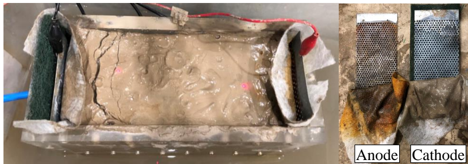
Figure 7.6 Test 1 using pure electro-osmosis and steel plate as electrode
