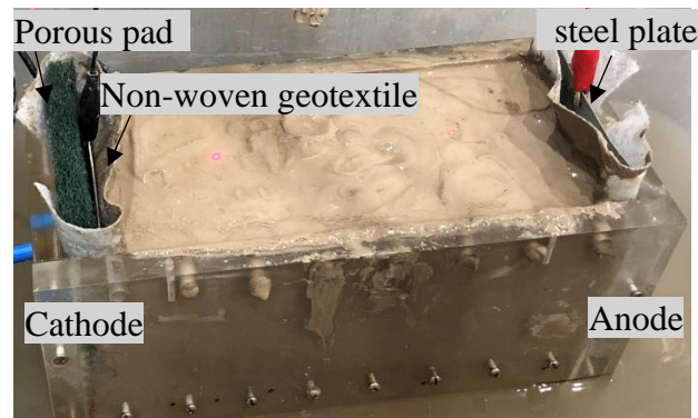
(a) Using steel plate as electrode (Test 1)
