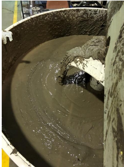
Figure 5.3 Mixed marine clay slurry used for the model tests
