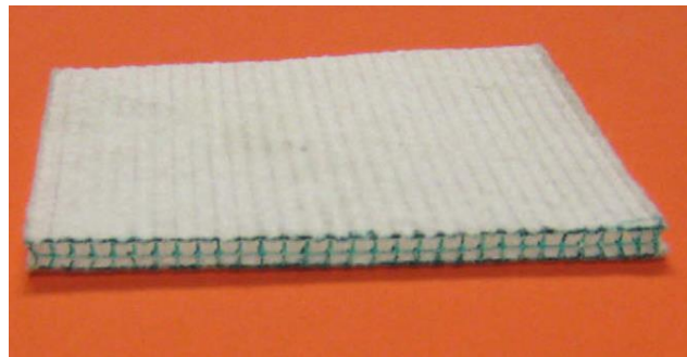
Figure 2.7 Integrated prefabricated drain (after Liu and Chu, 2009)
