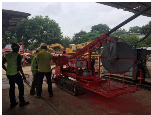
Figure 2.8 Installation sequence of PVDs ( https://www.tencategeo.asia )
