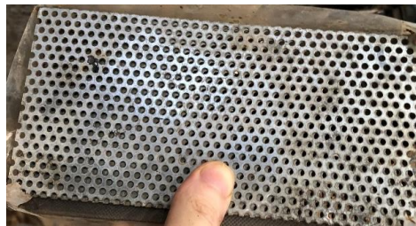
(a) Steel plate with round holes (thickness: 1mm)
