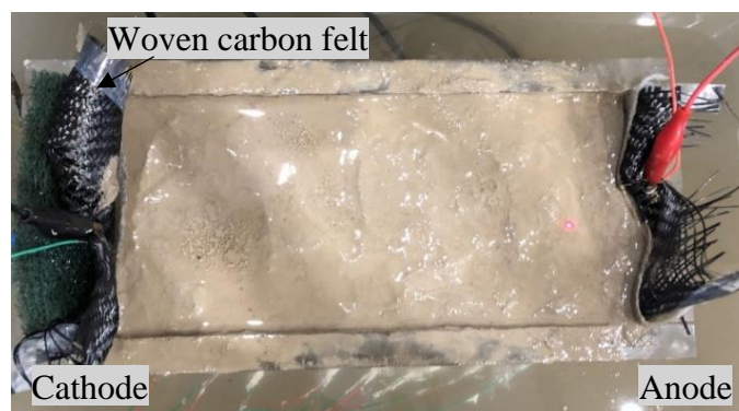
(b) Using carbon felt as electrode (Test 2)
