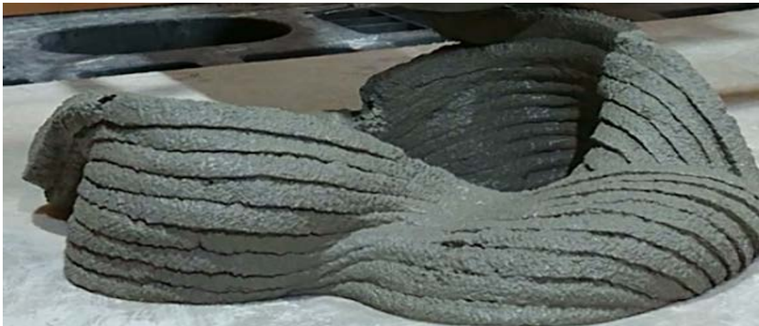
455 Fig. 12 Failure printing with material selected out of the optimum area (only 9 layers)
