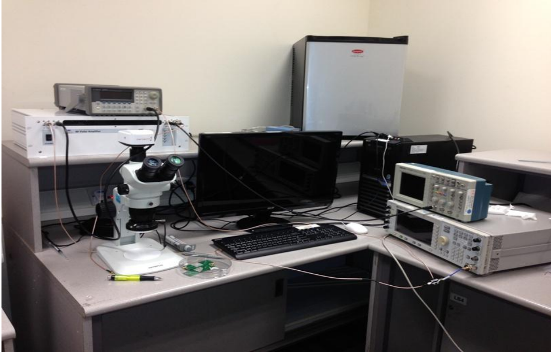
Figure 59: SAW pumping test setup.
