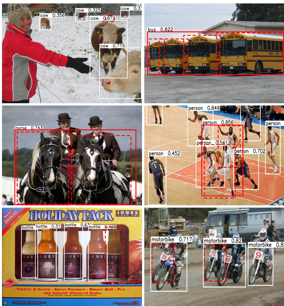
FIGURE 5.9: Visualization of some failure cases of Meta-DETR’s 10-shot object detection results. For simplicity, only detections of novel-class objects are illustrated. White boxes indicate true positives. Red solid boxes indicate false positives. Red dashed boxes indicate false negatives.
