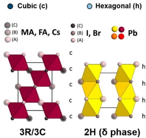
Figure 5: FAPbI 3 perovskite cubic and hexagonal (or delta phase) structures. Schematics reproduced from reference [41].
