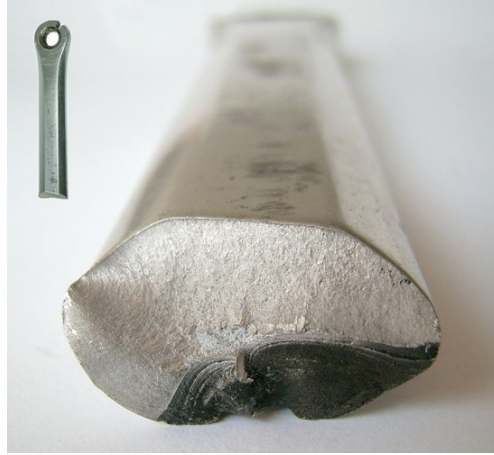
Figure 2.6. Cross-section of a failed aluminum crank arm
