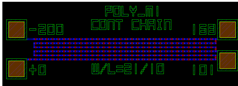
Fig. B-5 Contact chain between GPoly and METAL1.
