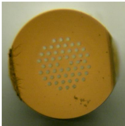
Figure 40: Microscope image of the LMA-25 photonic crystal fiber cross section. Cladding diameter is 268 \mu\text{m} for reference.
