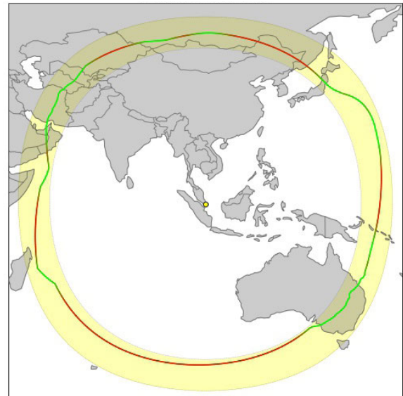
FIGURE 18. Isochrone with flight time of 7 hours to Singapore airport (green = data available, red = interpolation).
