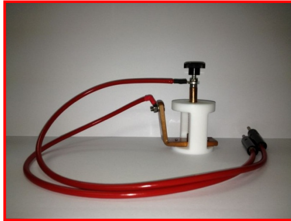
Fig 3.1 Customized in-house jig for ferroelectric testing.
