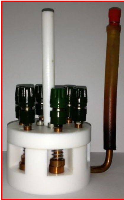
Fig. 3.2. Customized in-house jig for poling of multiple samples.
