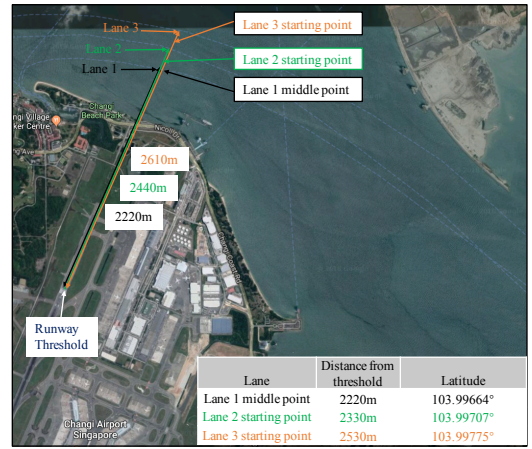
Fig. 6. Distance from the runway threshold and their corresponding latitude at the starting point of each lane. The picture and data are from Google Map.
