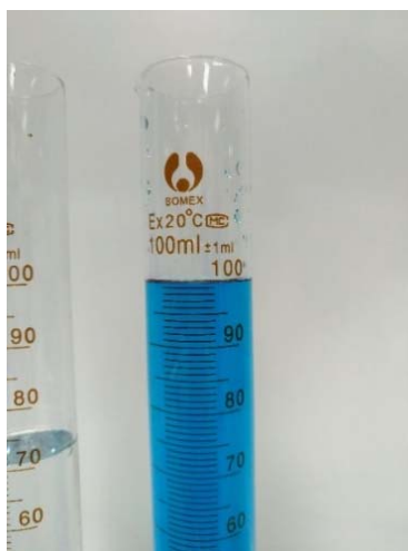
Figure S5. The image of the volume of blue dyed water after 5 times continuous oil-water separation test.
