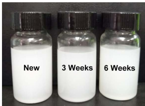
Figure S3. The imagines of the dipping emulsion after stored for different period times with volume radio for THF and water was 3:7.
