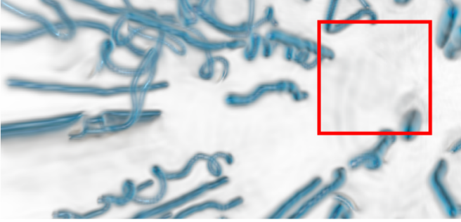
Fig. 15. By applying direct volume rendering, compression waves can be observed in the field magnitude. These waves, e.g., see the red boxed region, are energy releases from the vortex reconnections, and they accumulate by the transmission through the periodic boundary.
