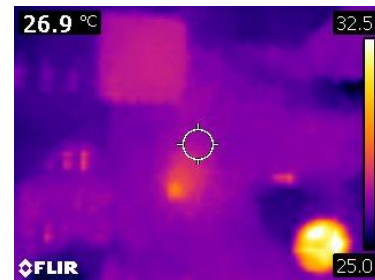
Fig. 9 IR image of the evaluation board top view after 30 mins operation.
