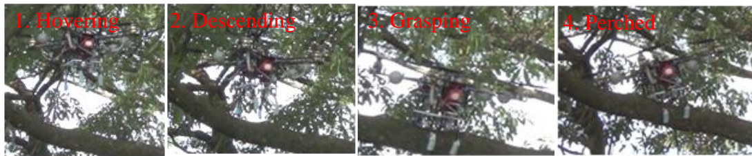
Figure 6.14 Perching to a tree branch (1: Hovering; 2: Descending; 3: Grasping; 4: Perched)
