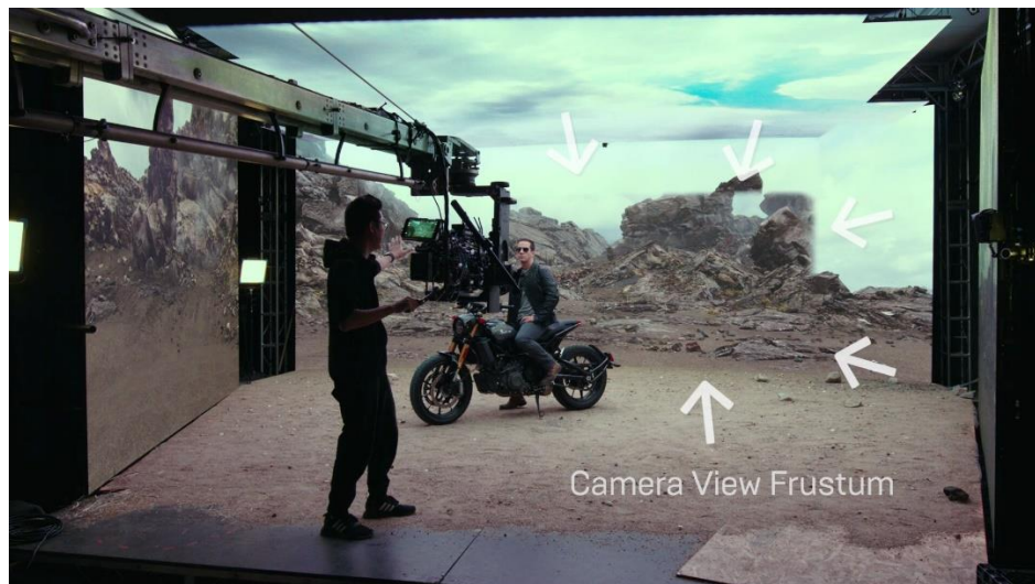
A Typical Setup for ICVFX: LED wall with Camera View Frustum
