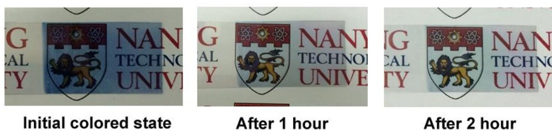
Figure 6.10. Demonstration of color memory effect of \text{WO}_3 film in air without voltage bias. The blue color is discernable for more than 2 hours.
