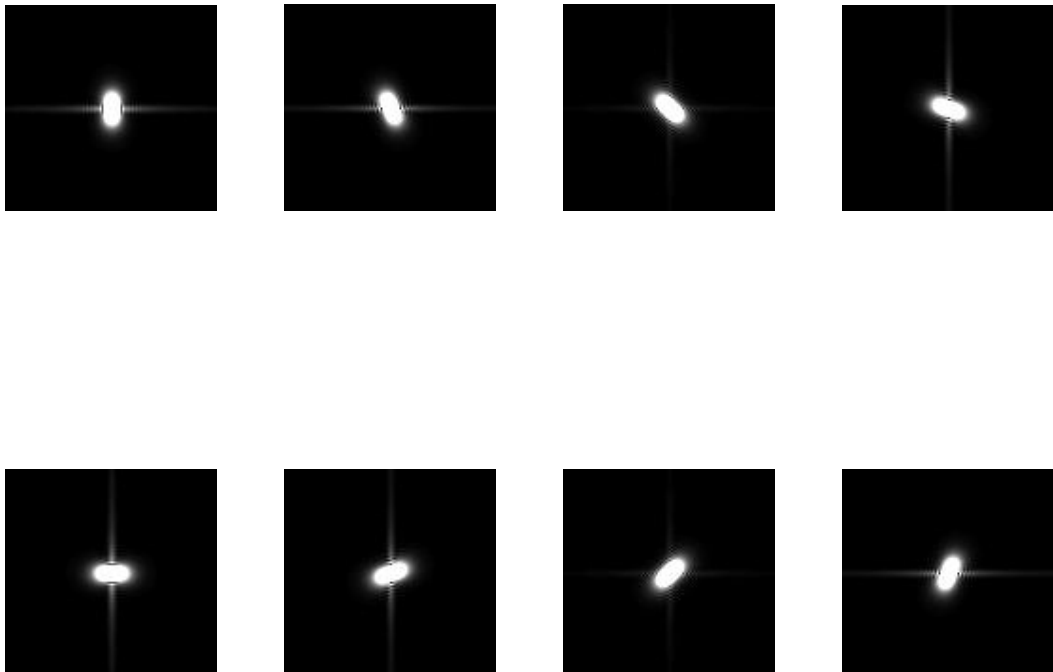
Figure 5.3: 2D log-Gabor filters at different orientations.
